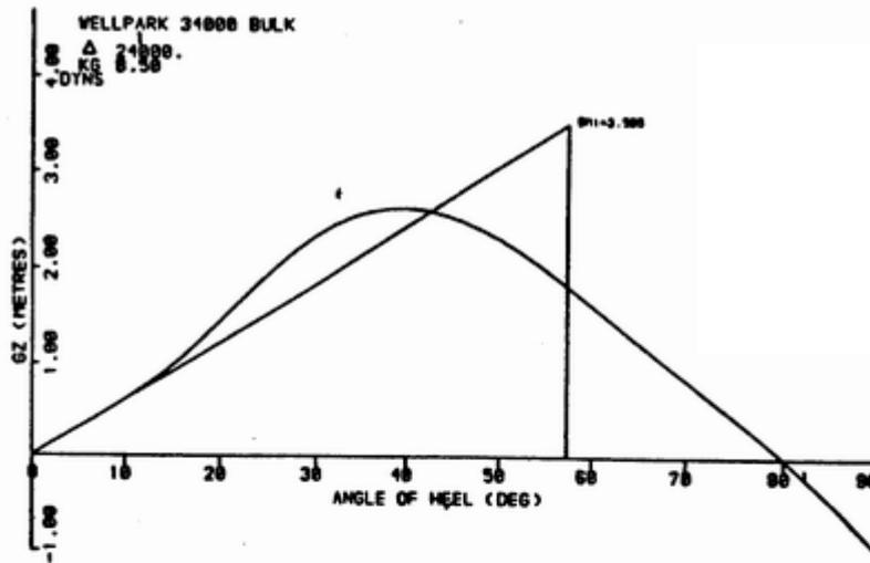
GZ CURVE OF A TYPICAL STABLE VESSEL
